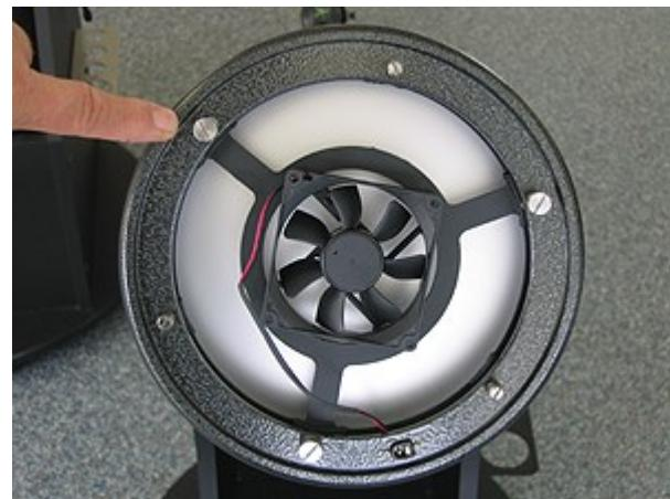
**Shows the collimation adjustment screws**
