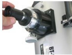
**Eyepiece being fitted to telescope**
