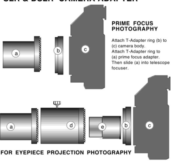
Attach (a) Prime focus adapter to
