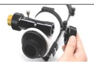
Remove the coarse adjustment knob of the telescope focuser using a suitable 1 sized wrench
