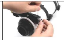
Install the flexible coupling on the telescope focuser shaft and tighten the lock screw
