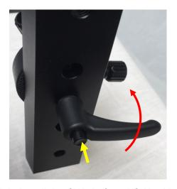
Install the mounting block back to the SkyTracker Pro and lock it. Install the CW shaft and CW, with larger bore facing to the safety lock.
