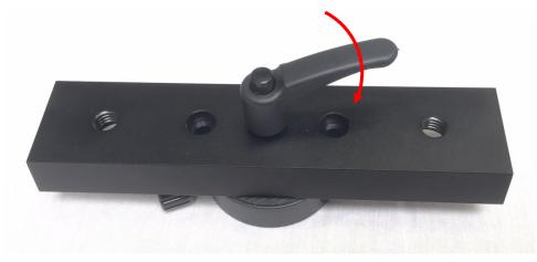
You can push down the center button and turn the lever without loosening the mounting screw. So you can put lever arm at any place you want.
