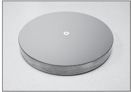
Figure 2. A center mark (ring) on a reflector's primary mirror greatly aids in collimation.
